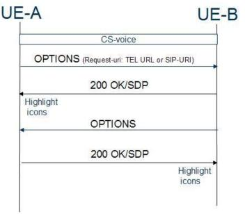
Figure 3: Capability Query using SIP OPTIONS
