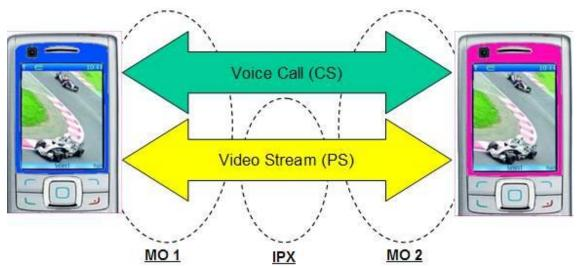
Figure 1High-Level Figure of Video Share Connection
