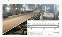
Sealing-tape machines are prone to motor or reducer failures, belt misalignments, slip, tearing, and other issues during production and operation due to the complex operating environment, the long transportation distance, and the large transportation volume. What's worse, the lack of effective detection and monitoring methods can lead to consequences ranging from lowered production efficiency to severe accidents.
