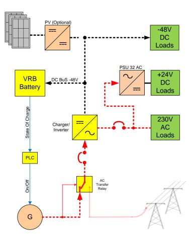
If the energy from the VRB<sup>™</sup> drops below predetermined SOC level and the utility power is still unavailable (or not stable enough), the system controller will provide a command for the Generator to start. The energy flow will now be as per diagram below
