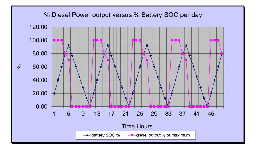
Generator run time savings are substantial if VRB<sup>™</sup> only charged to 90% of capacity. Charge time = 5 hours, Discharge time = ~ 5 ½ hours for a 4kW site load
