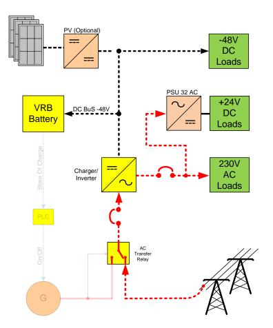
In normal operation the power is supplied from the utility grid. The AC power is channeled via Inverter/Charger to the loads and the battery is being charged, as per diagram below
