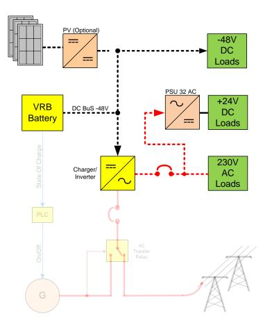
When the grid voltage drops below allowable limit, the Inverter starts generating AC power from the energy stored in VRB<sup>™</sup> Battery. This switch over happens within 8mS, short enough not to interrupt load operation. The power will continue to be powered from the battery per diagram above
