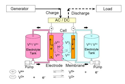
Vanadium forms stable, concentrated electrolytic solutions in four neighbouring oxidation states. The different states can be clearly identified by changing colours.
