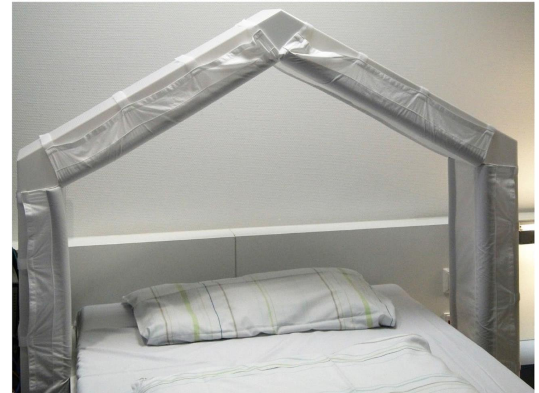
Fig. 2. Structure containing the antennas. Six commercially available Wi-Fi patch antennas were positioned every 60° along a circle of 0.6 m radius in order to meet the requirement of an almost uniform exposure of the head regardless of the subject's position. Danker-Hopfe et al, IJHEH, 2020
