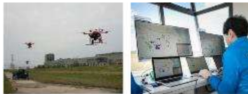
Simultaneous control of up to 37 units by large-scale drone control system
